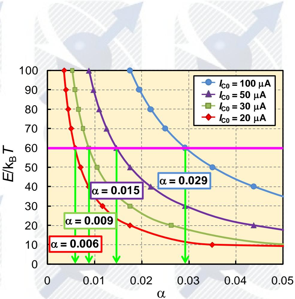
$$I_{C0} = 3.4 \times 10^3 \alpha [\mu\text{A}] \text{ for } E = 60 k_B T$$
