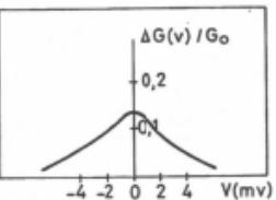
Fig. 2. Relative conductance  $(\Delta G/G)_V=0$  of Fe-Ge-Co junctions at 4.2 K.  $\Delta G$  is the difference between the two conductance values corresponding to parallel and antiparallel magnetizations of the two ferromagnetic films.
