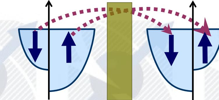
Ferromagnet 1      Insulator      Ferromagnet 2
